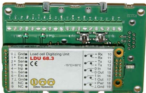
UA77.4 / 77.6 Board with screw terminals for I/O functions + 2 Input keys, and + LED for output indication RS232 or RS485 output
