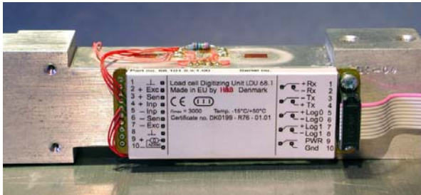
LDU can be supplied only with soldering holes as shown here
