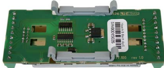
UA77.1 same type as UA73.3 but mounted with RS422 to RS232 converter as shown on the PCB.
