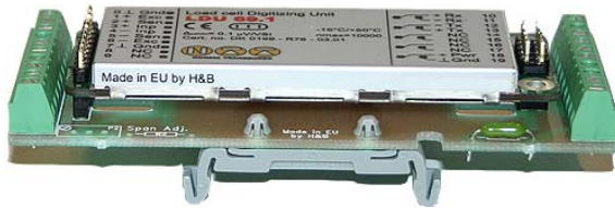
UA73.202 PCB for DIN Rail mounting with screw terminals and female sockets for LDU
