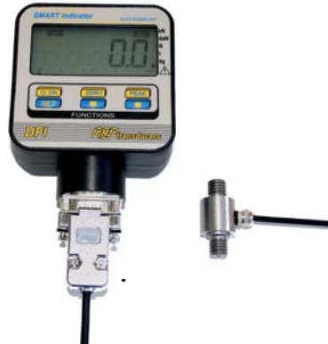
DFI battery based instrumentation
