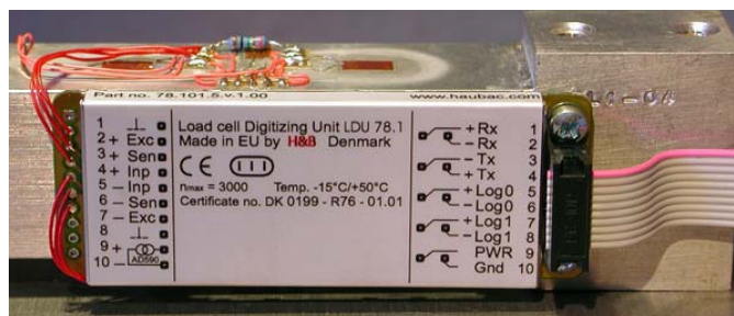
LDU78.1 OIML approved unit for fast checkweigher or filling machine jobs with up to 2400 updates/second at any mode, on command !
